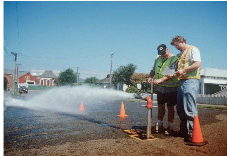
City Care staff testing fire hydrant water pressure
