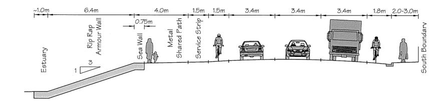
4.0m Shared Path with 3in1 Sloping Embankment Section
