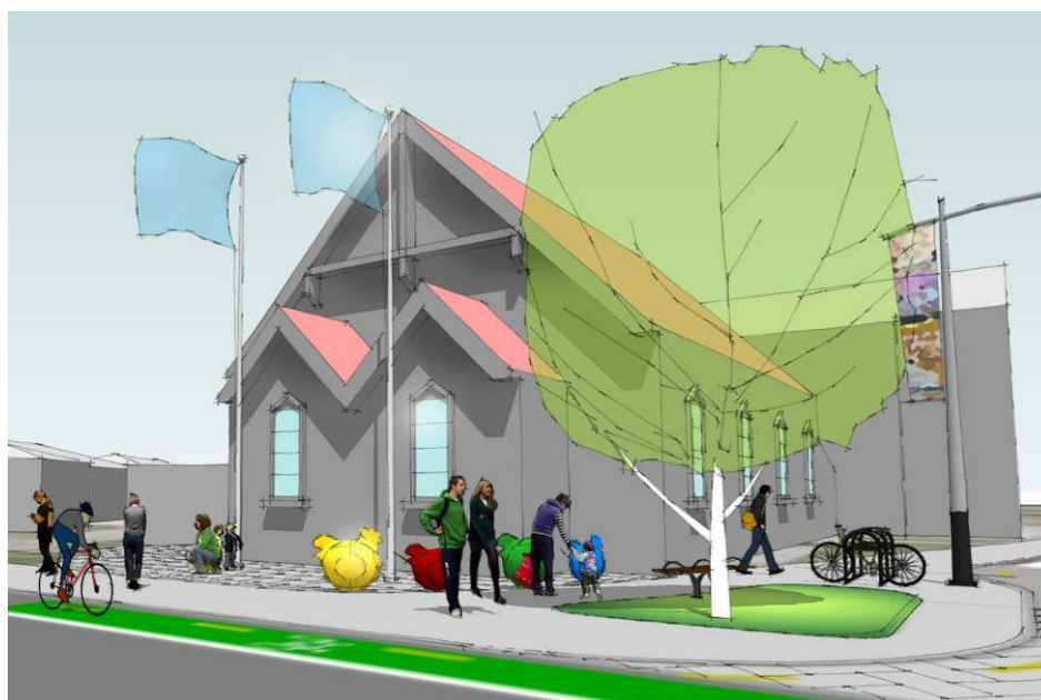
Figure 28. Artist's impression of the kerb extension and planting on the Corner of Selwyn Street and Somerset Crescent in front of the church hall
