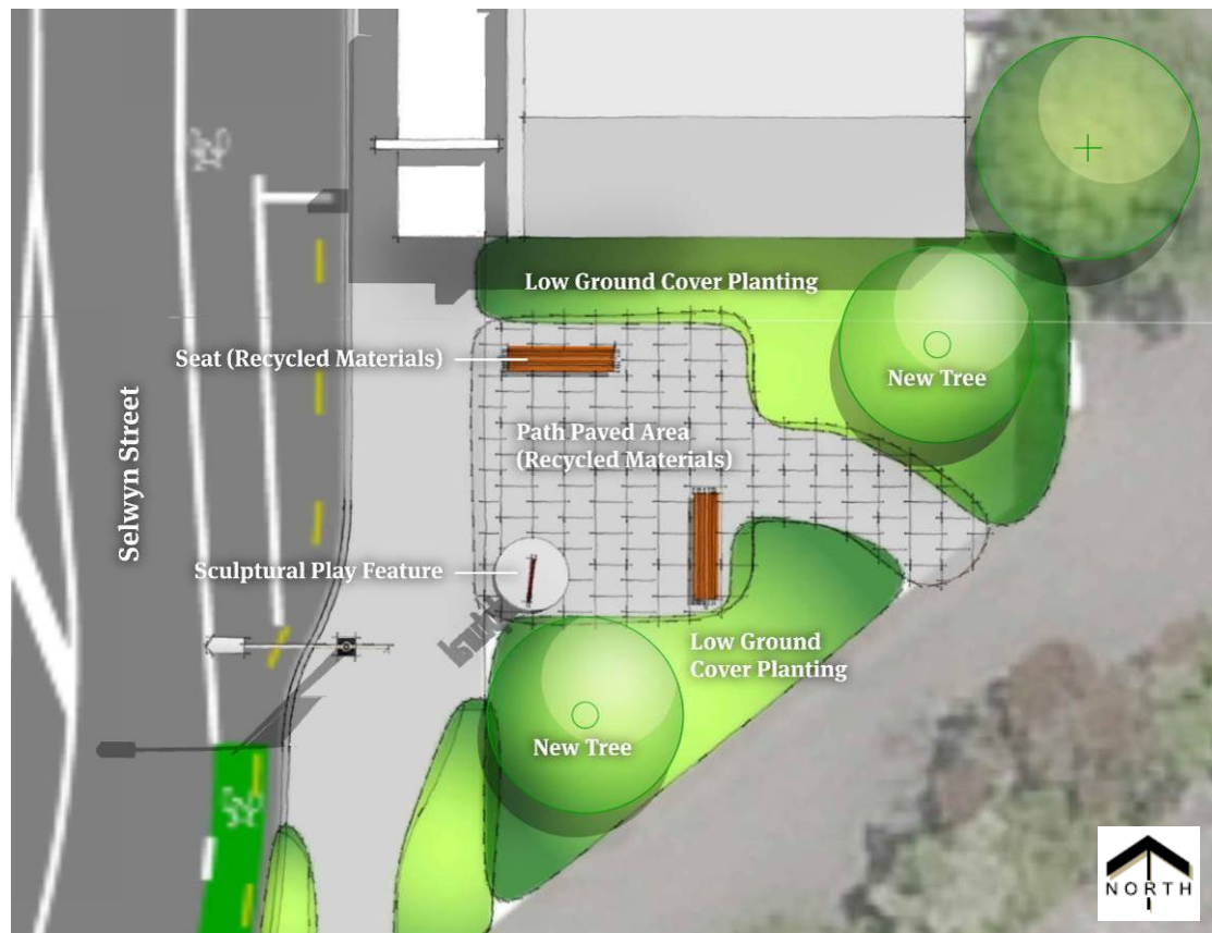
Figure 24. Concept plan of a seating area adjacent to 288a Selwyn Street, better utilising the space for the community on the frontage of the adjacent housing units
