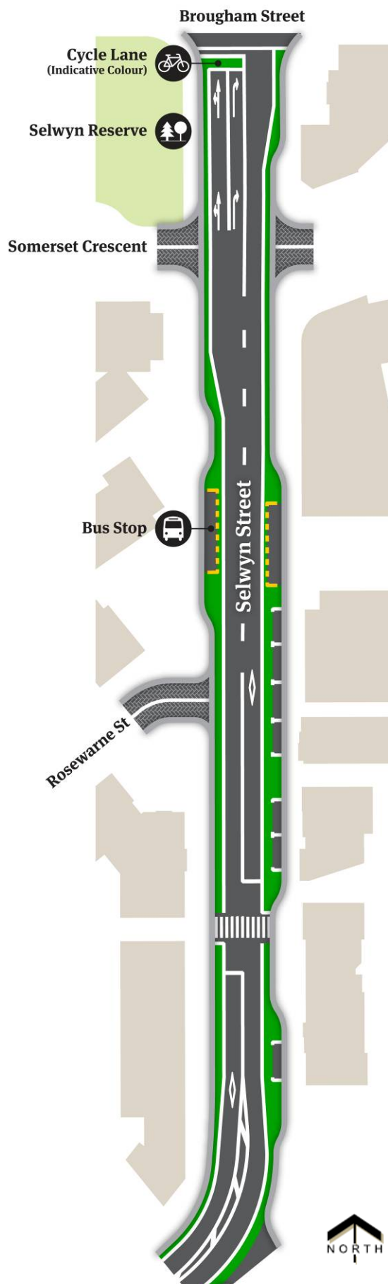
Figure 25. Proposed Street modifications (indicative drawing; solid green marking will not be continuous the length of the cycle lanes but will be used through and on the approaches to intersections and crossing points)
