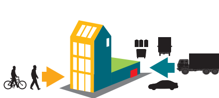
Fronts and backs serving different needs Parking and servicing located at rear Limited vehicle accessways
