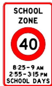
Figure 3 Fixed 40 kilometre per hour Variable Speed Limit Sign – as used in Christchurch
