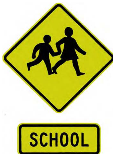
Figure 7: Fixed School Warning Sign
