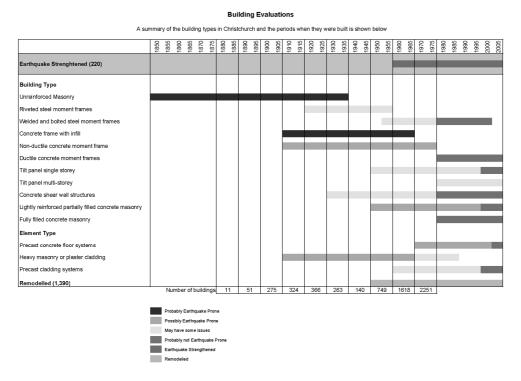
**Unreinforced masonry** - 1860 to 1940s. The highest risk construction method. Floors and roof generally light timber framed. Cost of strengthening typical building \$350-450/m² to 33% FCL (full code level).
