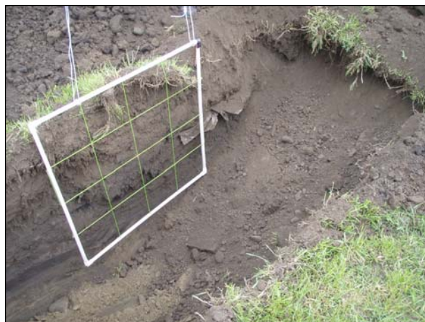
Photograph 3: View of the soil and waste material within test pit TP4
