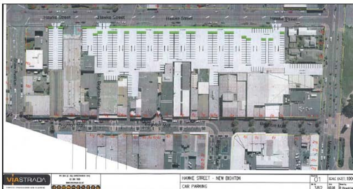
Figure 15: Hypothetical Redevelopment of Hawke Street (two access points only, approximately 380 car parks)
