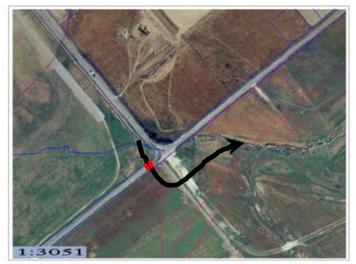
This proposal includes diverting the watercourse to cross Wigram Road via a new culvert West of the intersection with Haytons Road and reconnecting it to the existing waterway upstream of the Proposed Southern Motorway extension. The access way into the A&P showgrounds will need to be renewed with a ford (with low flow piping underneath the ford). In the event of a flood access can be re-routed west of the waterway onto Wigram Road.
