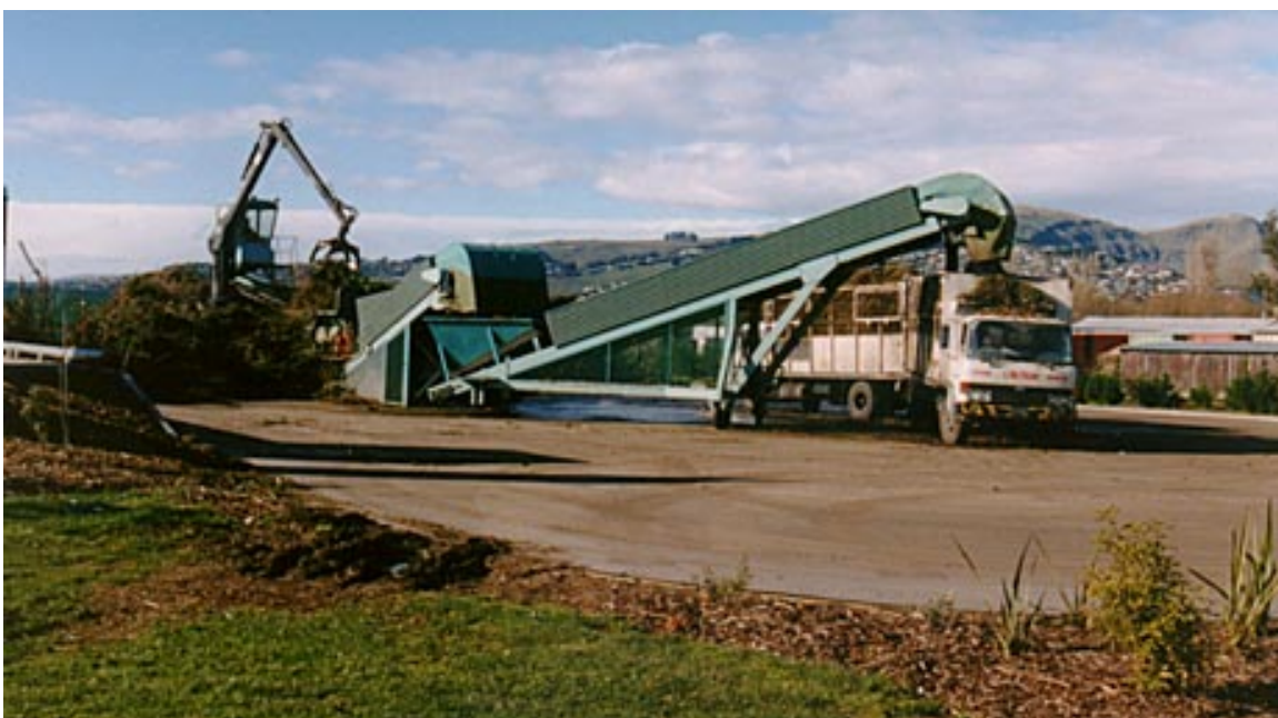
Green waste being processed by the Shredder at the Metro Transfer Station.
