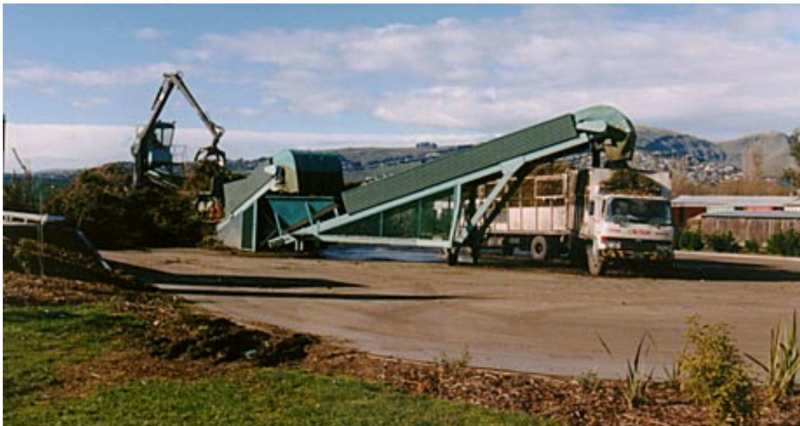
Green waste being processed by the Shredder at the Metro Transfer Station.
