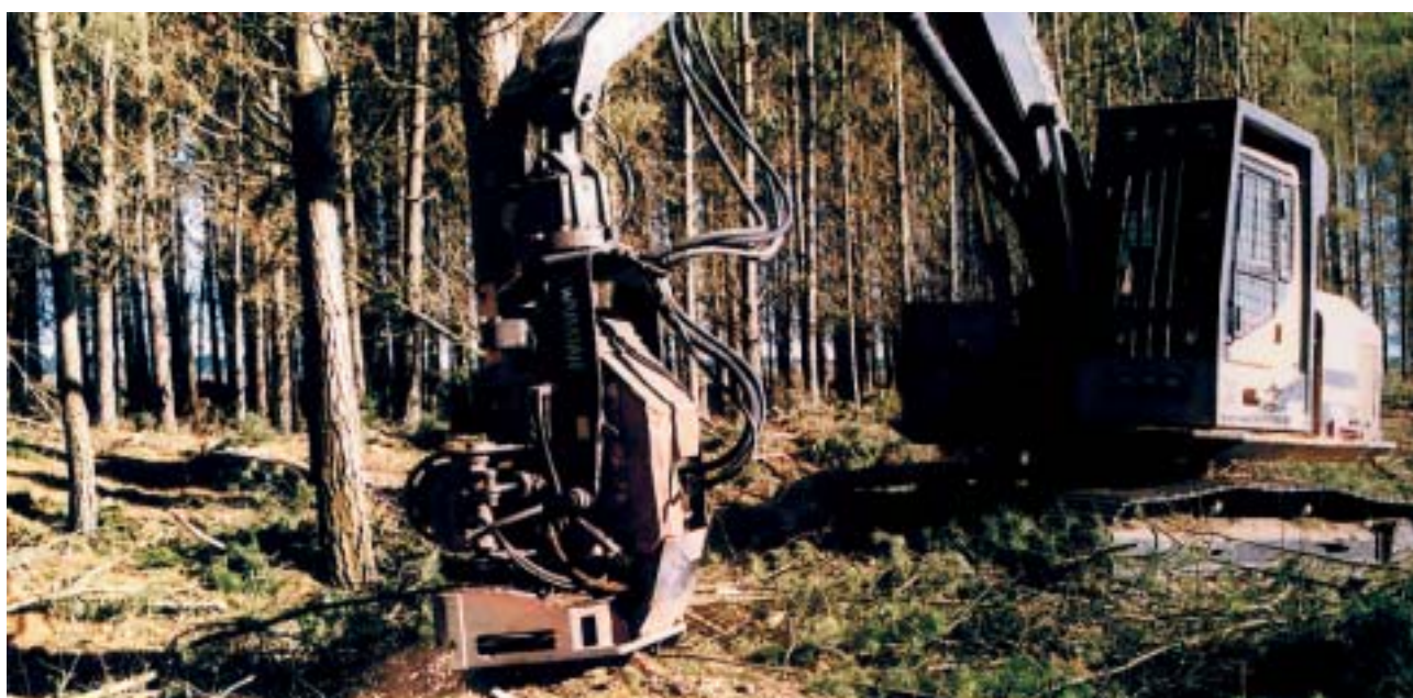
A Waratah whole tree harvester being used to fell trees in the Southbridge Plantation.
